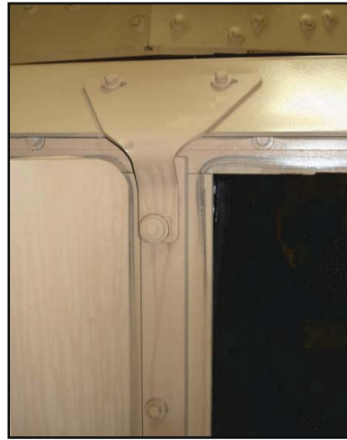
(U) Figure 7. Bolt-on B-Pillar of the M1151
