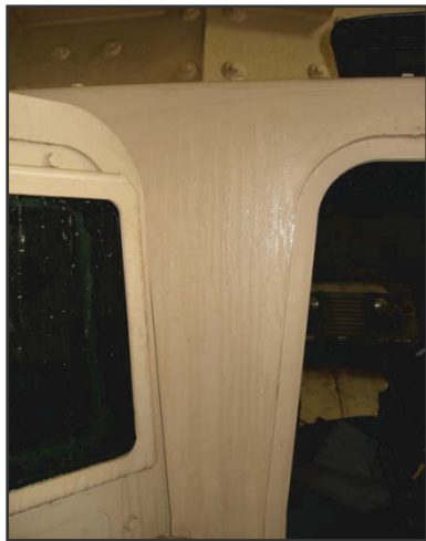
(U) Figure 6. Welded B-Pillar of the XM1166
