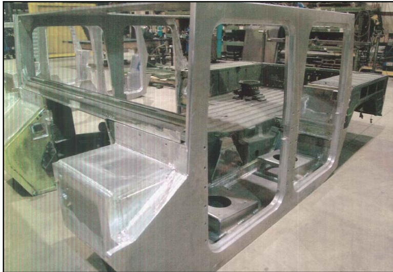
(U) Figure 8. Welded Cab of the XM1166
